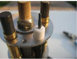
Once the Spring Clip is removed, slip the igniter out of the top washer as shown at right.
