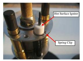
Remove the Spring Clip using a Spring Clip Removal Tool as shown at right.
