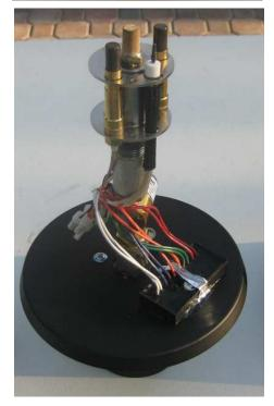
At right is a close up of the burner section of the Tiki Torch. Notice the Hot Surface Igniter is held in place by a spring clip.
